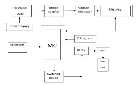
Figure 1: Block diagram of the operation processes and design methods of the UCB
